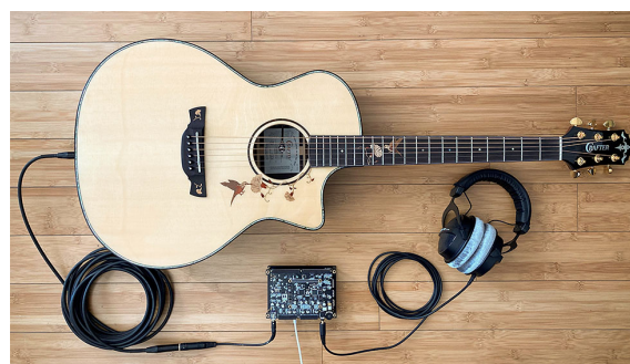
Figure 1: Hardware setup of the expressive technique classifier. The audio signal from the guitar pickup is fed to a Raspberry PI through the Elk PI Hat, which contains high definition audio converters. The result of the classification is communicated through a simple sine wave tune with different frequencies, which is monitored with a pair of headphones.
