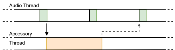
Fig. 5. Representation of a digital audio system with a more relaxed real-time constraint than those of Fig. 2 (i.e., not audio-rate deadlines) where some costly computations must be performed less frequently than calls to the audio callback and can be conducted on a separate thread. This can be the case of event-based DL inference [15], where signal analysis is performed only when events are detected. In these cases, event detection is a less costly operation performed for each audio block, while the heavier analysis is allowed to take more than the time budget for a single audio callback call.
